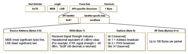
Bytes 5-6 contain the source address. An MI6/SPECTRE should ignore the packet if the source address does not match the address they stored as being the paired device.
